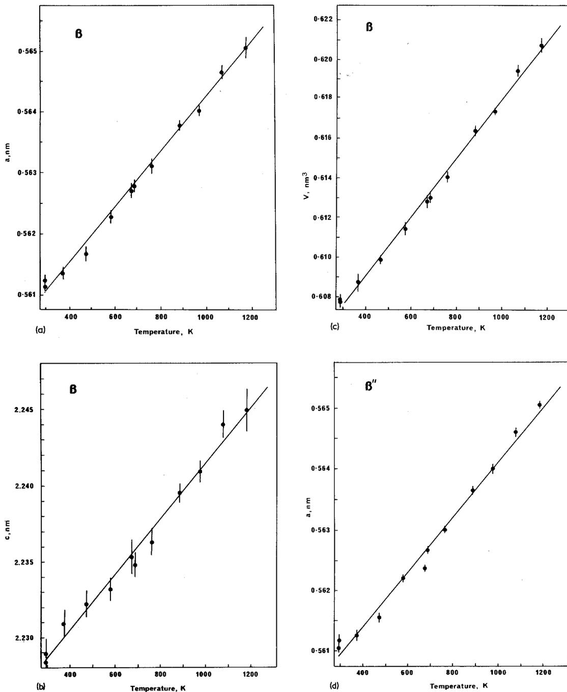
Figure 3 Variation of  $a$ ,  $c$  and  $V$  cell parameters of  $\beta$ - and  $\beta'$ -alumina with temperature. Data plotted are marked with asterisks in Table II. The error bars are for one standard error. The lines were computed by least squares.
